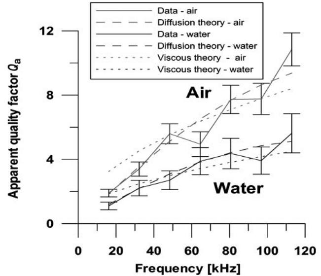
Figure 3. Apparent quality factor  $Q_a$  versus frequency, for air-saturated (red color) and water-saturated (blue color) cases. Experimental values obtained for a 40-mm layer (solid lines) are compared with a theoretical diffusive-viscous model (dashed lines) and a purely viscous model (dotted lines).
