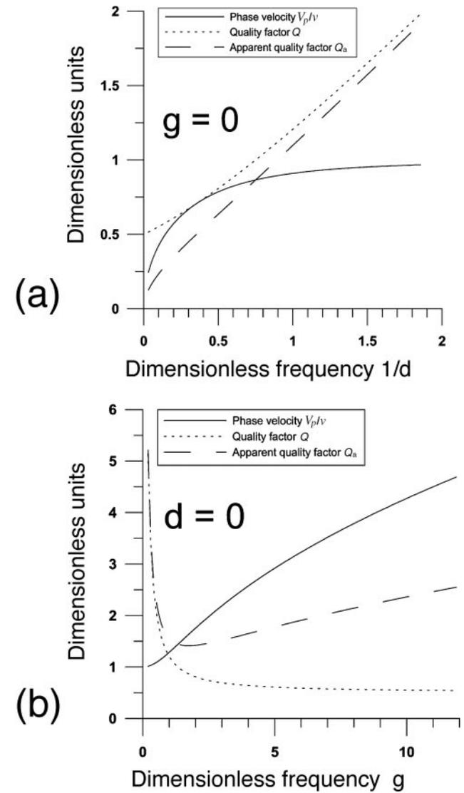
Figure 4. Normalized phase velocity  $V_p/v = \omega/kv$  (solid line), attenuation factor  $Q$  (dotted line), and apparent attenuation factor  $Q_a$  (dashed line) as functions of nondimensional frequency for (a)  $\gamma = 0$  and (b)  $\chi = 0$  cases. All three quantities are dimensionless and plotted on the same vertical axis.
