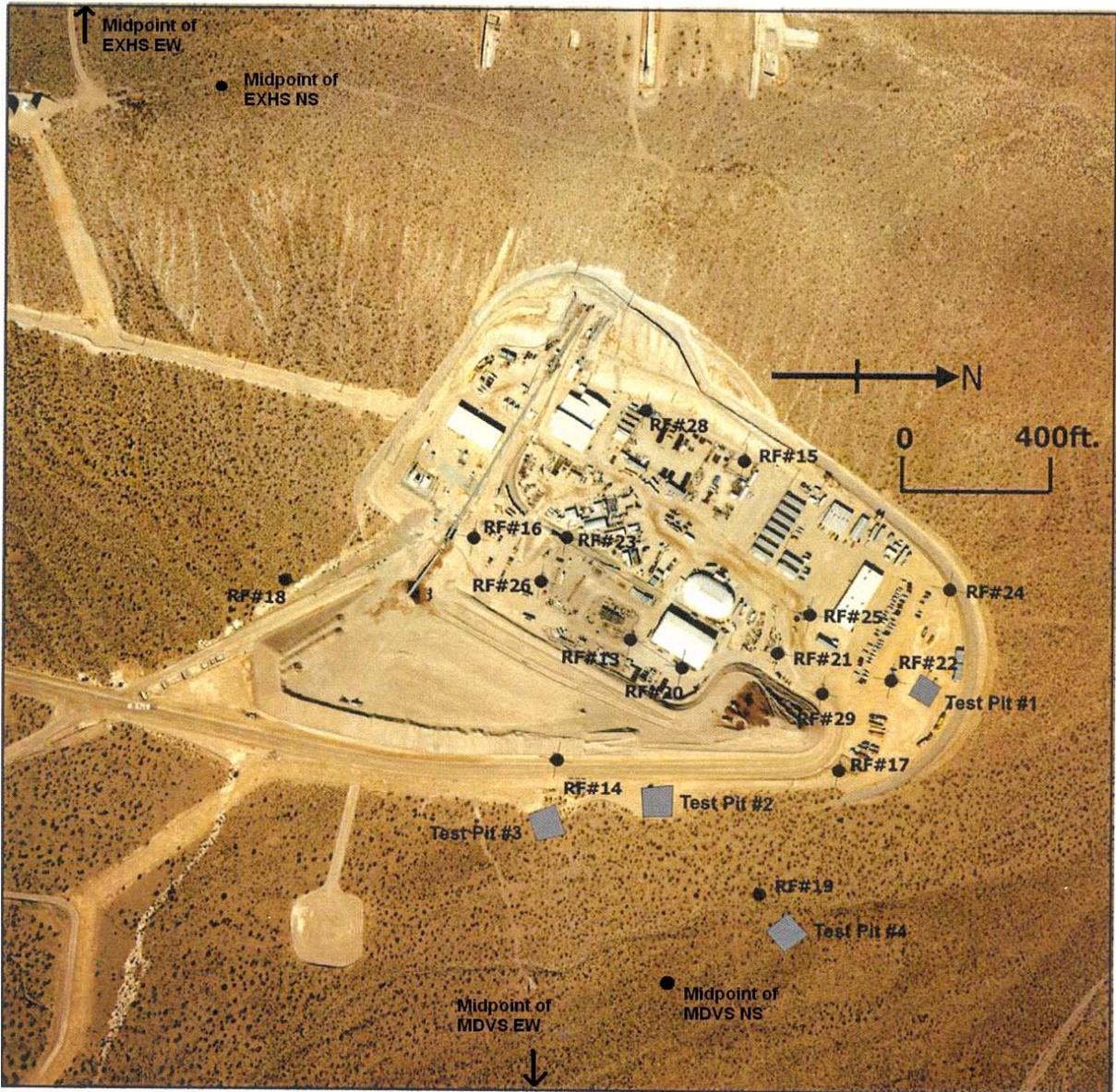
Figure 4. Map of the Yucca Mountain Tunnel Entrance pad from Luebbers et al. (2002), modified to show ReMi measurement sites MDVS and EXHS. The midpoint of the MDVS EW array is ~200 ft (60 m) east of eastern map edge (bottom). The midpoint of the EXHS EW array is ~200 ft west of the western map edge (top), following the road.
