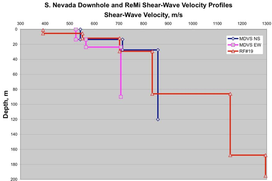
Figure 6. Profiles of shear-wave velocity versus depth of ReMi site Midway Valley and borehole site RF#19 in southern Nevada. RF#19 was the borehole measurement taken nearest, within 300 m, to both Midway Valley array center points.
