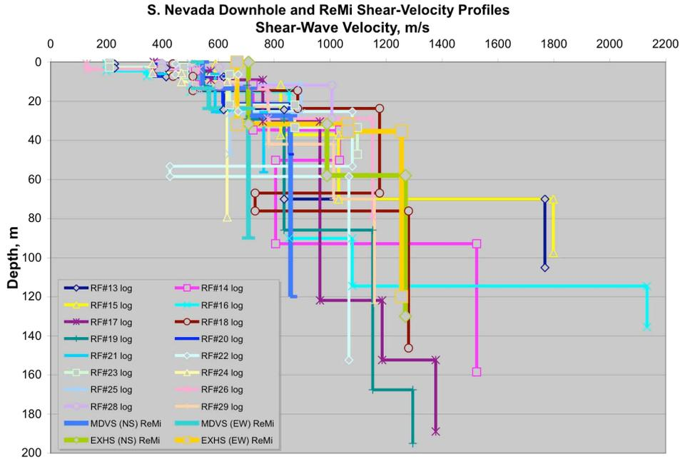
Figure 5. Shear-wave velocity profiles from the downhole and ReMi measurements examined at the Yucca Mountain Tunnel Entrance pad in southern Nevada (Figure 4).
