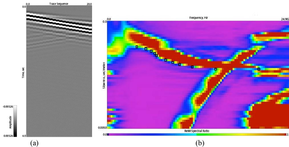
Figure 2. (a) Four seconds of example 20-trace E3D synthetic-seismogram record from a model array extending 285 m. (b) Example image of slowness-frequency ( $p$ - $f$ ) spectrum. The warmer colors of the image represent increased spectral ratio in the manner of Louie (2001); the ratio of spectral power at a particular  $p$  and  $f$  over the average spectral power for all slownesses at that  $f$ . The small squares indicate analyst's picks of the fundamental-mode Rayleigh-wave phase velocity.
