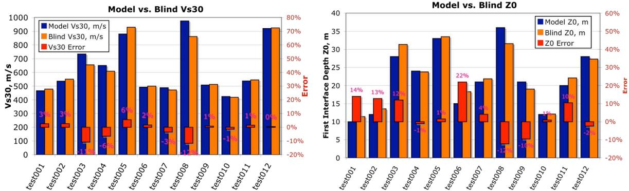
Figure 3. Comparisons of original-model Vs30 (left) and Z0 (right) against corresponding results from blind ReMi analyses of synthetic data records.
