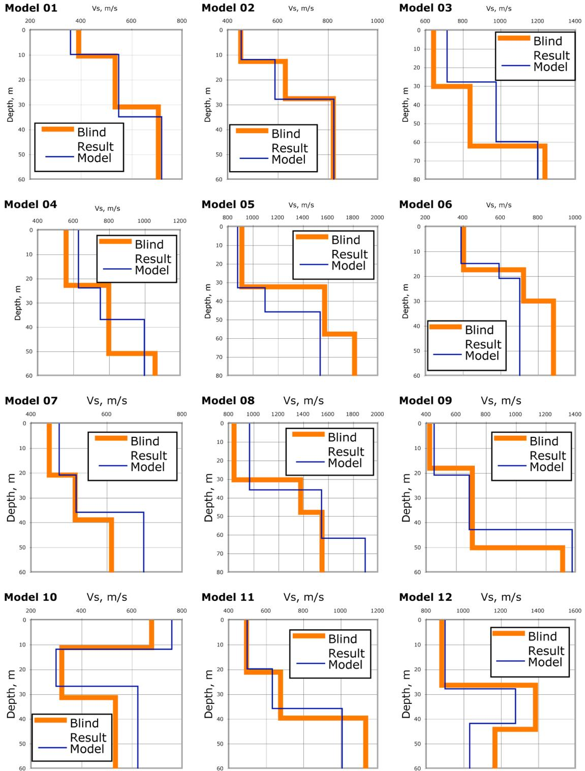
Figure 1. Model shear-velocity versus depth profiles for the synthetic ReMi analyses. Ten of the twelve profiles represent Sheriff's (1991) A-type section of increasing velocity with depth. The remaining two profiles correspond to an H-type section and a K-type section. The H-type section (Model 10) has a low-velocity layer, while the K-type section (Model 12) has a high-velocity layer.
